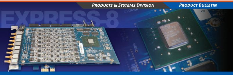
MISTRAS' Acoustic Emission data acquisition board and system live up to their name. The EXPRESS-8 is a faster, more powerful AE system than its predecessors, fusing a PCI-Express bus with higher channel density and capabilities.
