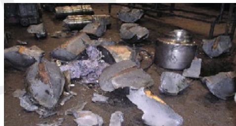
Catastrophic Roll Failure
