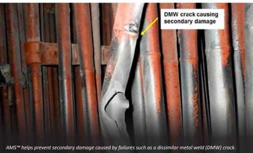
MISTRAS | Triple 5 offers technical support through Surveillance, a remote monitoring service that analyzes the data for acoustic changes and hardware issues. A report is sent on the status of the system by email to a group designated by the plant. A phone call is placed to the main contact and/or the control room when immediate attention is needed. A 24 hour hotline is available for high signal consultations after
